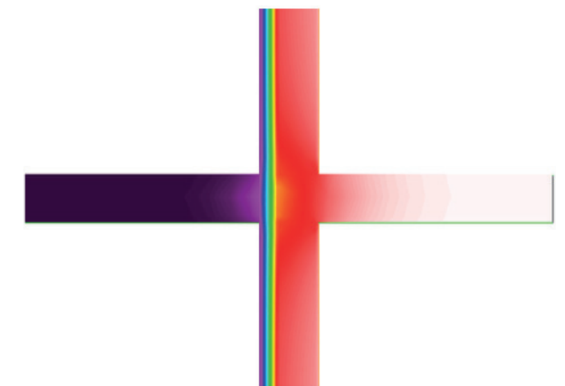
Figure C2: Simulated Temperature Profile of Exterior Insulated with Rigid XPS Insulation (R-15) Steel-Frame Wall Assembly at Thermally Broken Balcony Detail with 3-inch CIS Thermal Break
